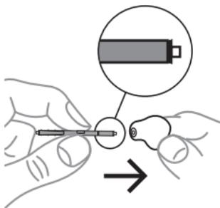
Insert the new wax guard into the opening of the sound outlet and press it gently.
