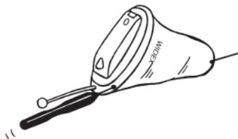
Long vent: clean the vent every day by passing the long wax removing tool (no. 3) all the way through the vent.
