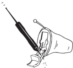
Open the battery lid and turn the hearing aid so the lid is facing downwards (see illustration). Guide the short wax removing tool (no. 4 ) through the microphone openings on the lid from the inside (see illustration).
