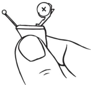
Use the nail grip to gently swing the battery door open and remove the old battery.
