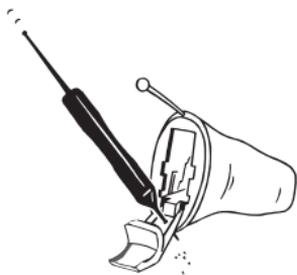
Short vent: clean the vent as far as the long end of the wax removing tool (no. 3) can reach.
