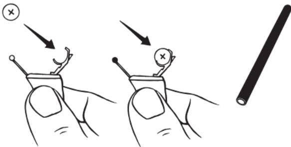
Close the drawer. If it doesn't close easily, the battery is not placed correctly.
