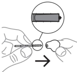
Insert the removal hook into the used wax guard.
