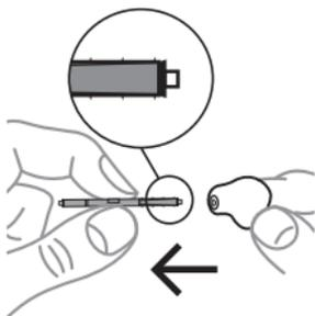
Pull the used wax guard straight out.
